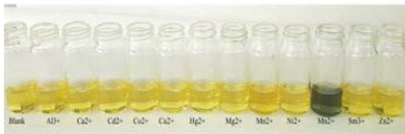
Figure 4. Photograph of the AgNPs in the absence and presence of 1 \mu\text{M} concentrations of the various metal ions.
